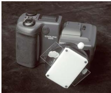
Figure 2. Film and transparency copying apparatus screwed on to lens of digital camera. The section, secured by Blue Tack, has been placed in a compartment between the camera lens and a white diffuser. Low power photomicrographs of high quality can be prepared by this method.
