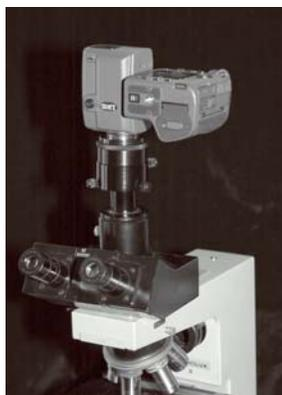
Figure 3. Digital camera attached externally to microscope eyepiece of central tube by adaptor which is screwed to thread on camera lens.
