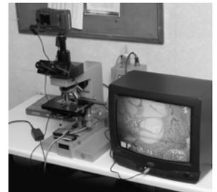
Figure 1. Microscope with digital camera mounted onto central tube through an adapter. The TV set is connected to the camera and, by showing the image and data depicted on the camera monitor in real time, becomes a useful large monitor for focussing.
