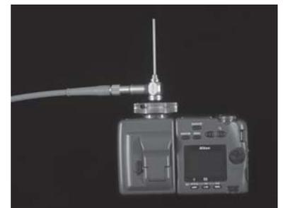
Fig. 4. Digital camera mounted to Hopkins rod with light source for digital otoscopic photography.
